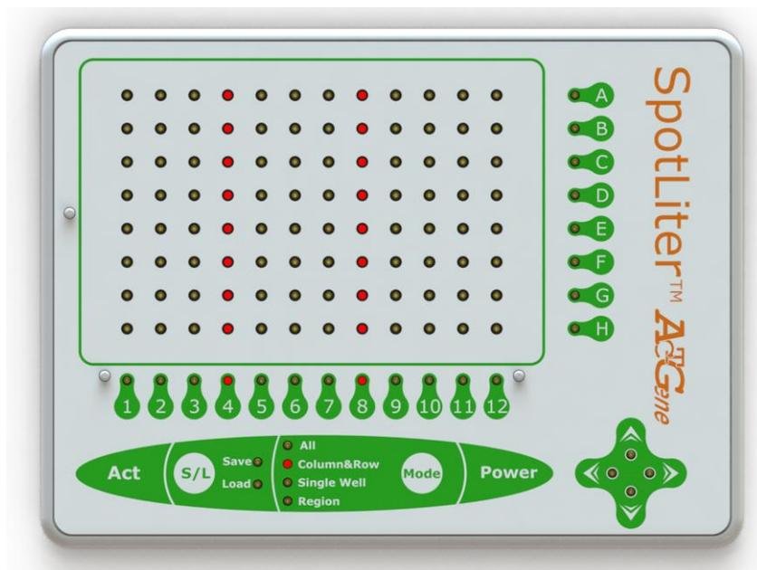
When switching to “Column & Row” mode, the direction control panel located on the bottom right corner will illuminate. At this time, any column or row can be selected, but column and row can’t be selected simultaneously. After selection, the direction control panel will be off. Pressing “Act” button or stepping on the foot pedal, the selected column or row will illuminate in selection order and one by one.
