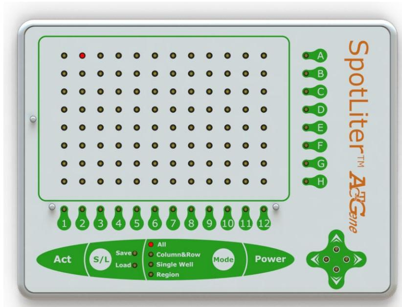
“All” mode is a default mode. Under “All” mode, only the “Act” button, foot pedal, and “Mode” button function. When pressing “Act” button, or stepping on foot pedal, the LED light will illuminate one by one. Press “Mode” button to switch the mode.
